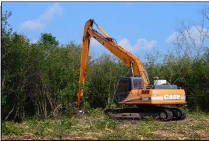
Chopper/grinder operated by Dennis Marshall reduces glossy buckthorn to wood chips.
